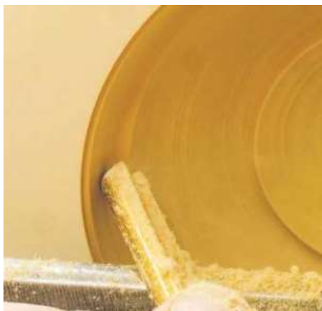
▲ Pic.28 I like to finish the inside of the bowl in stages. I use the 6mm bowl gouge for all the finishing cuts until the overhang becomes too great and causes vibration
